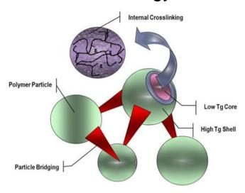
High Tg shell and low TG core facilitates film formation and strength in final coating
